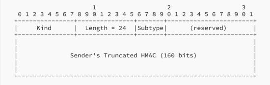
Figure 7: Join Connection (MP\_JOIN) Option (for Initiator's First ACK)
