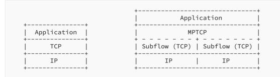
Figure 1: Comparison of Standard TCP and MPTCP Protocol Stacks
