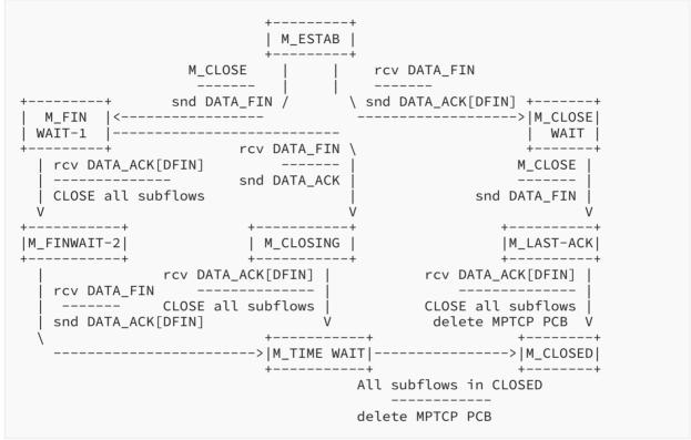
Figure 22: Finite State Machine for Connection Closure
