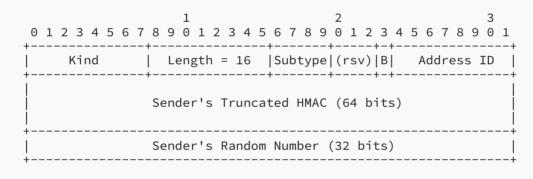
Figure 6: Join Connection (MP\_JOIN) Option (for Responding SYN/ACK)
