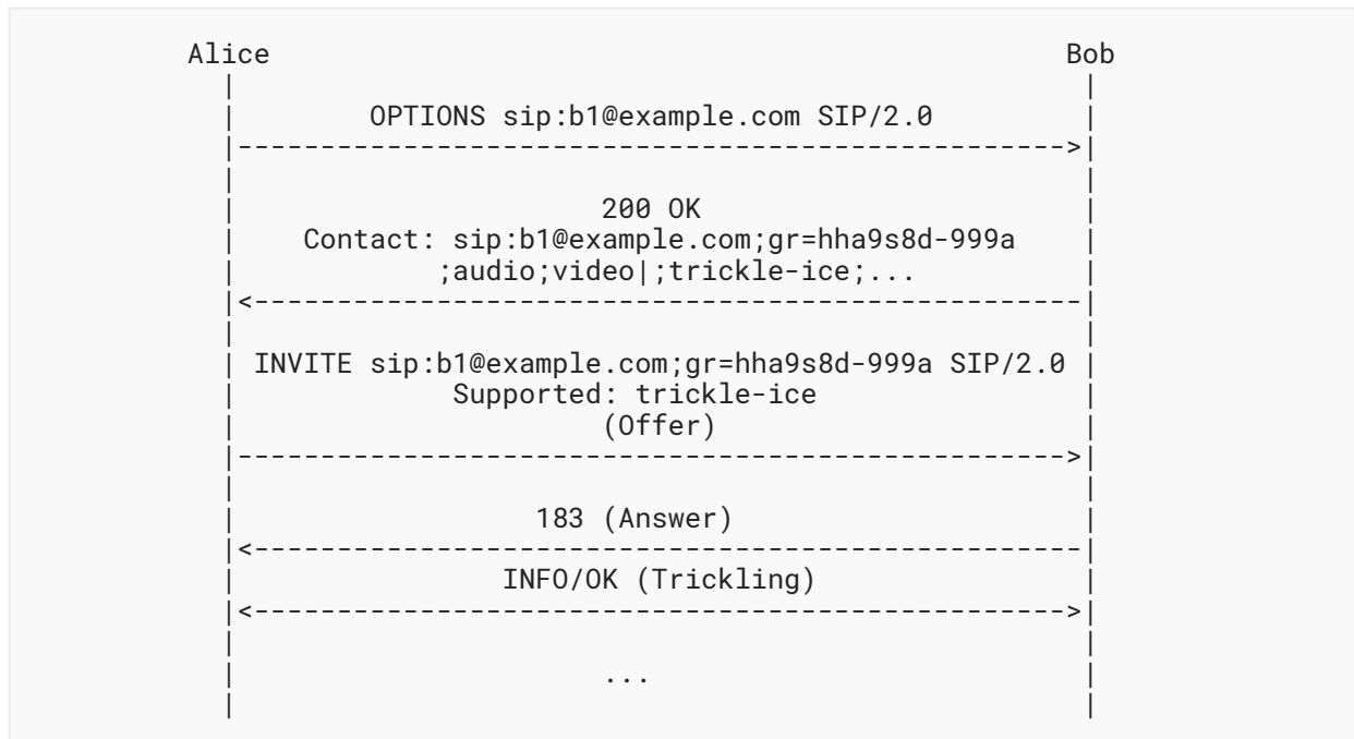
Figure 8: Trickle ICE Support Discovery with OPTIONS and GRUU
