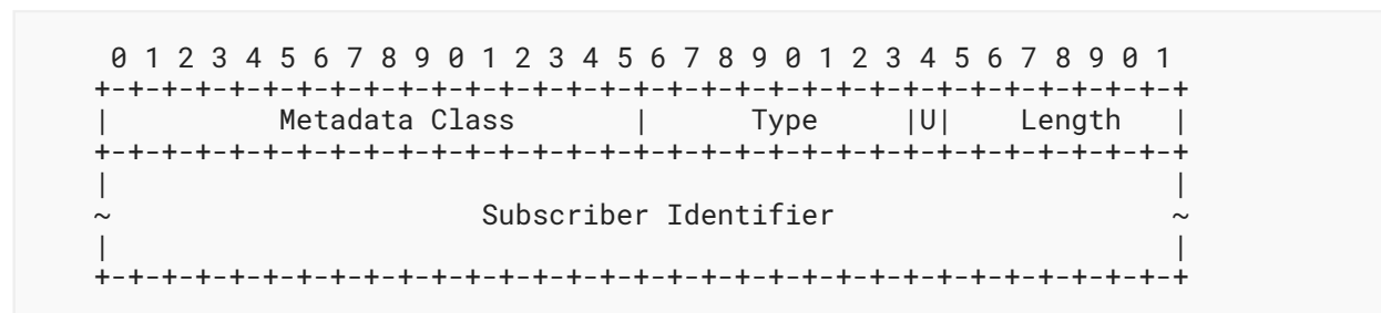
Figure 1: Subscriber Identifier Variable-Length Context Header
