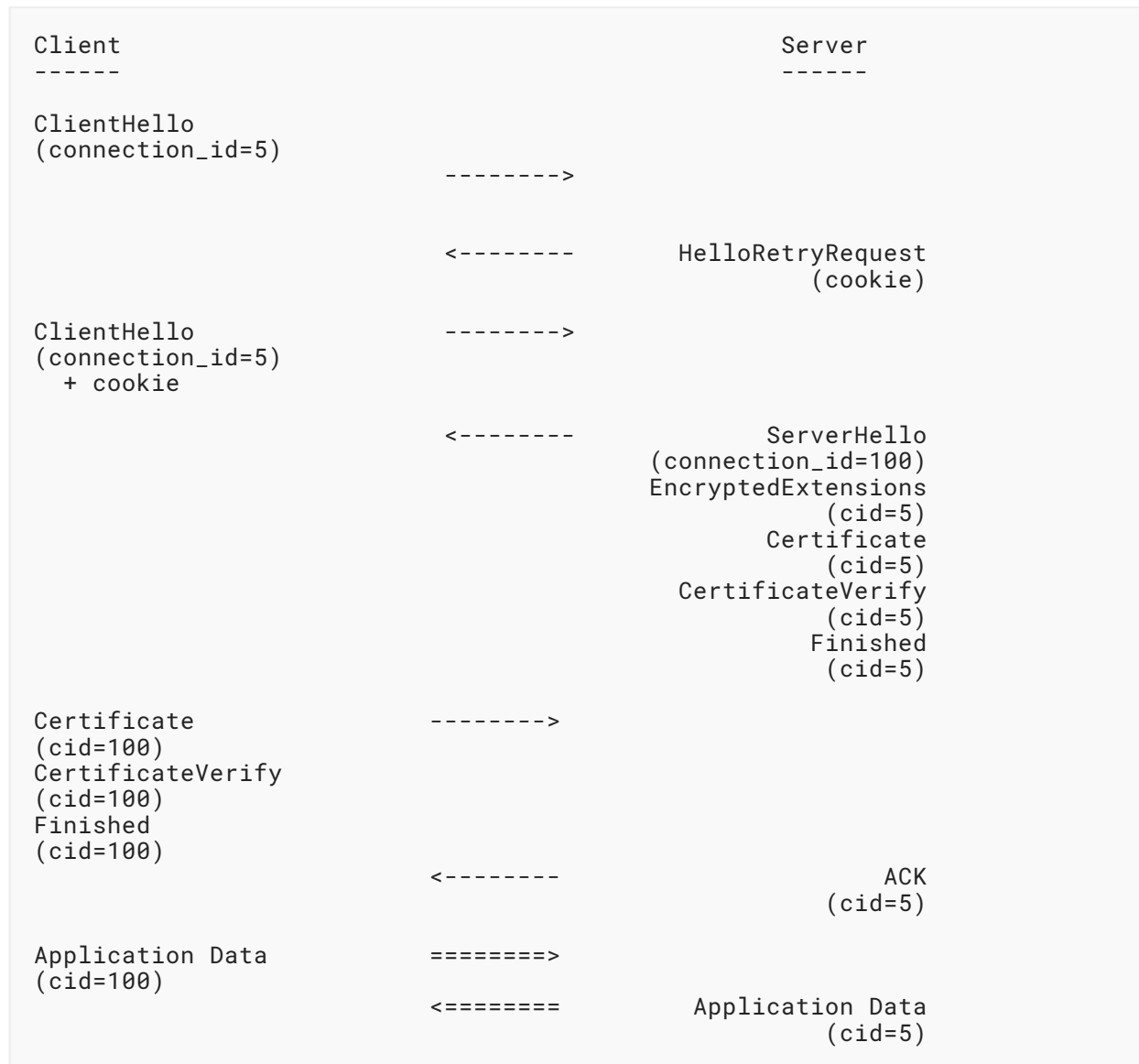
Figure 15: Example DTLS 1.3 Exchange with CIDs
